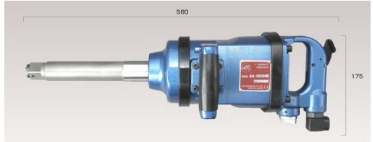
Heavy duty 1" Impact Wrench with 9" long anvil Single pinless hammer clutch, 3-step speed regulator
